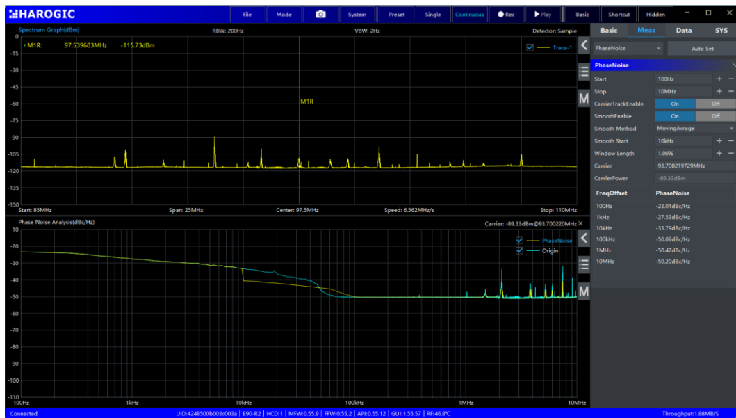
Figure 6 Phase noise analysis in SWP mode.
